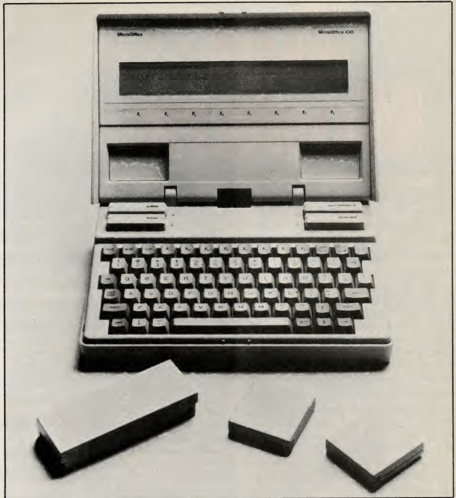
The MicroOffice RoadRunner opened up. In the foreground are a battery pack and two memory cartridges.
